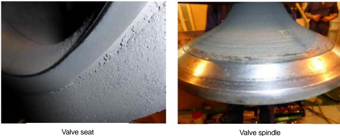
Figure 3: Photo from test vessel (G70ME-C9)
