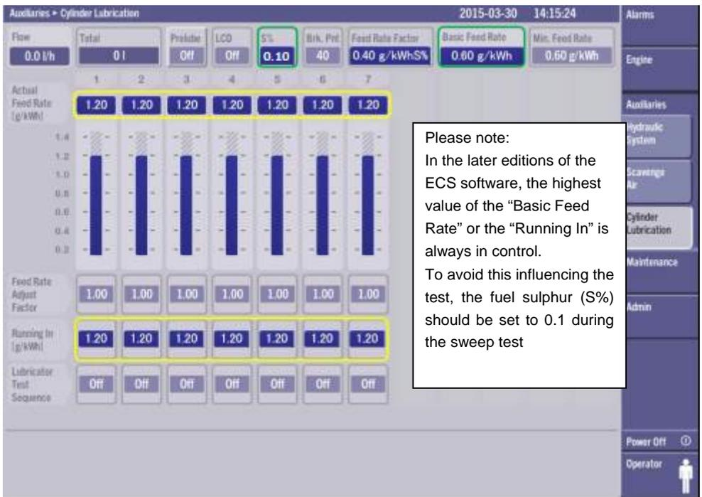
Figure 5. Day 2 of sweep test. The Running In mode is used and set to 1.2 g/kWh in this case the "Basic Feed Rate" is lower and the "Running In" is in control.
