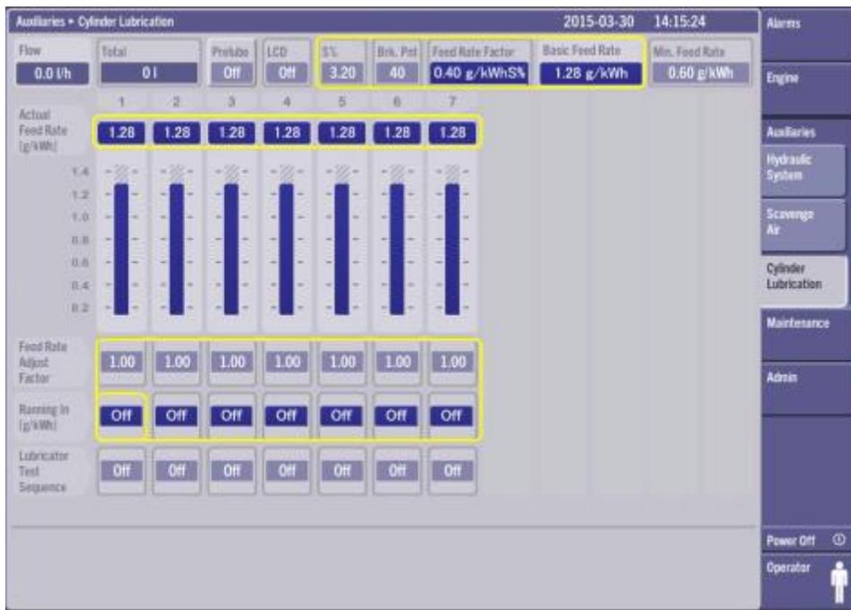
Figure 2. MOP-screen showing settings at normal running conditions. Running-in mode is turned OFF
