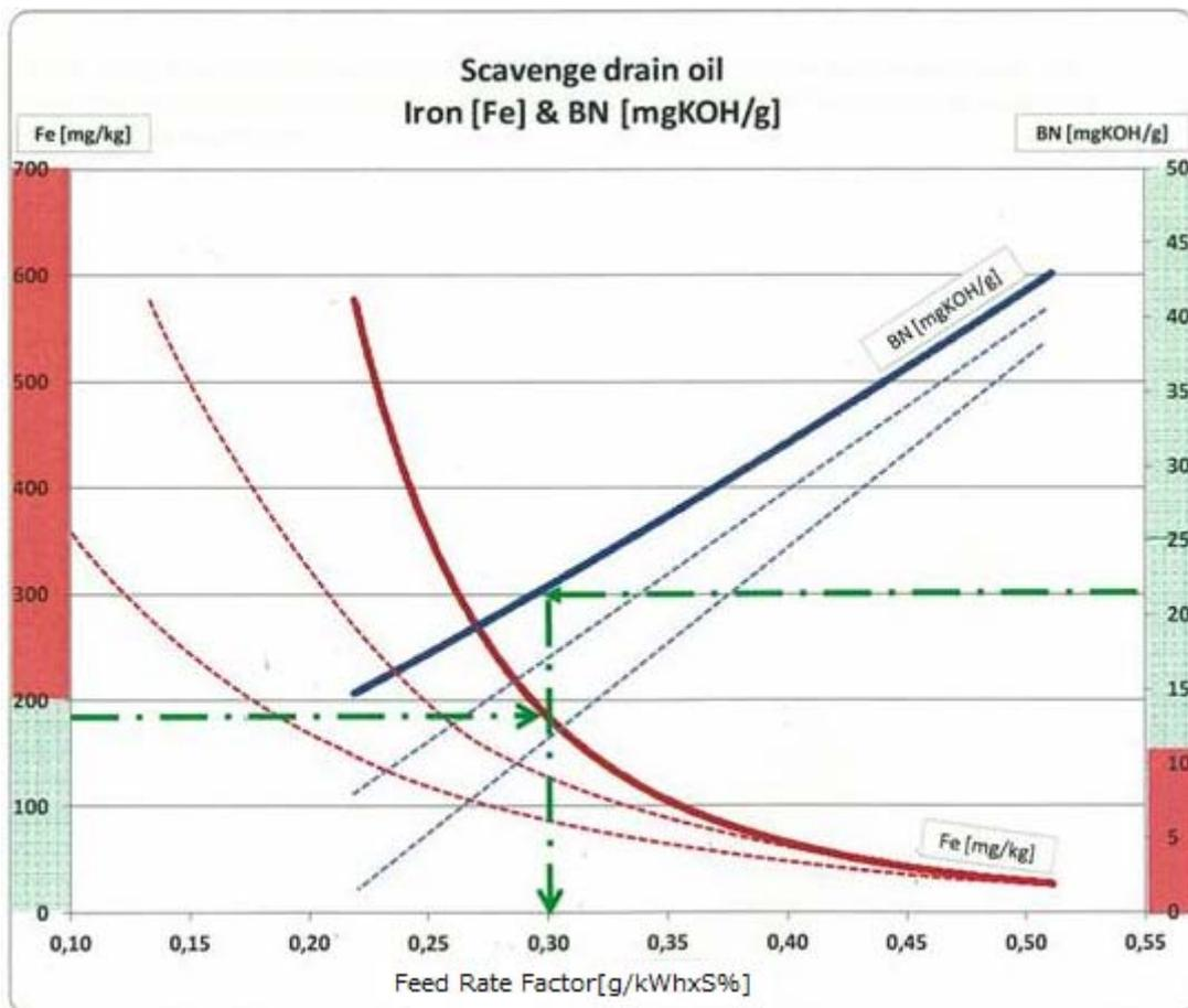
Figure 6. The Feed Rate Factor (g/kWhxS%) is shown on the x-axis. The Fe concentration (mg/kg) is depicted with red lines and the result is read on the left y-axis. The axis is divided into three parts. The green bar shows safe operation condition, 0-200 Fe (mg/kg). When the Fe concentration exceeds 200 mg/kg (the red bar), the wear or corrosion starts to increase significantly, and the lube oil feed rate should also be increased.
