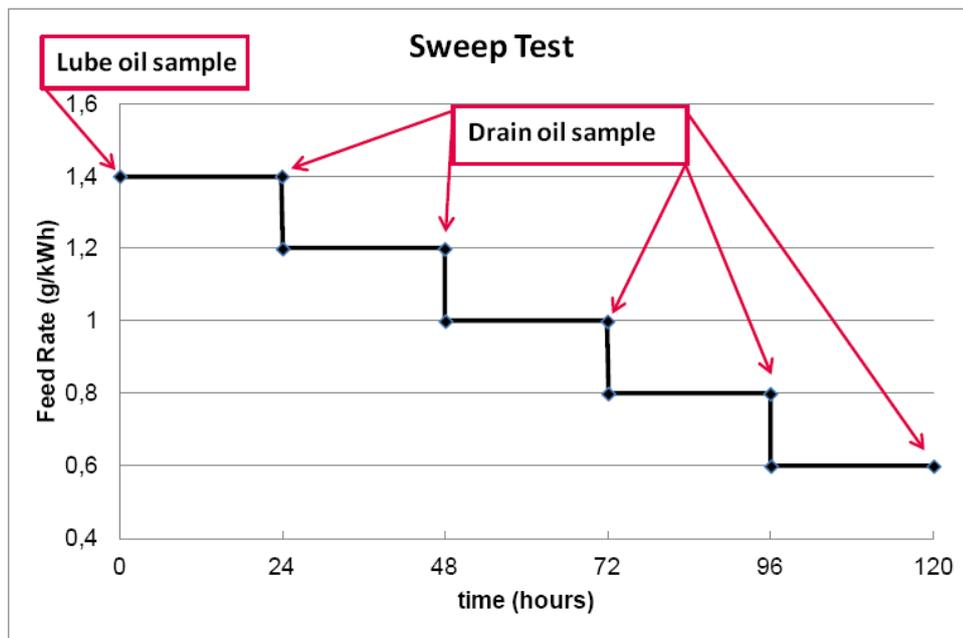
Figure 1. Overview of the sweep test procedure
