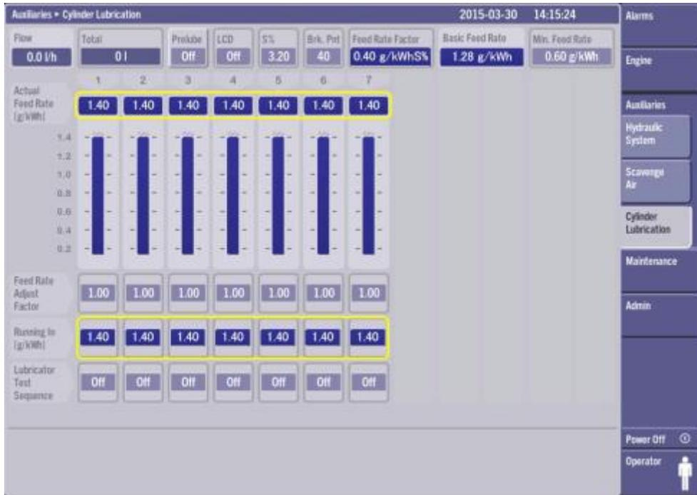
Figure 3. Day 1 of sweep test. The Running In mode is used and set to 1.4 g/kWh
