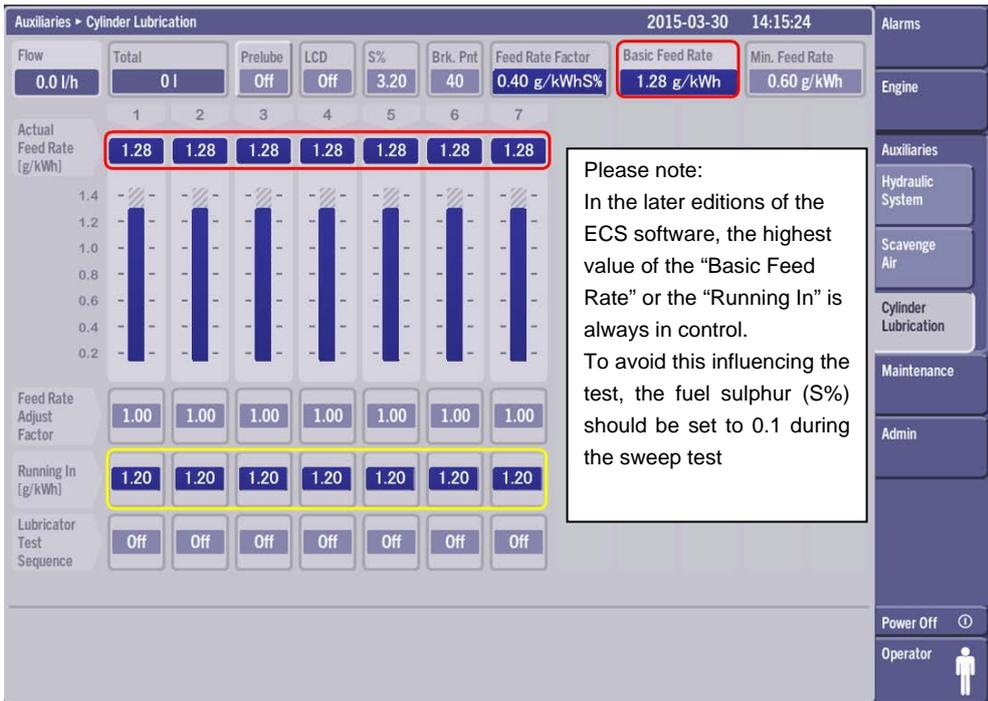
Figure 4. Day 2 of sweep test. The Running In mode is used and set to 1.2 g/kWh, and in this case the "Basic Feed Rate" is higher and over-rides the "Running In".
